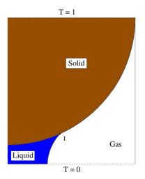
Fig. 3. Sketch of the cylindrical computational domain (taking into account all the symmetries). Boundary conditions are of homogeneous Dirichlet type on top and bottom sides, and of Neumann type on the external vertical side.
